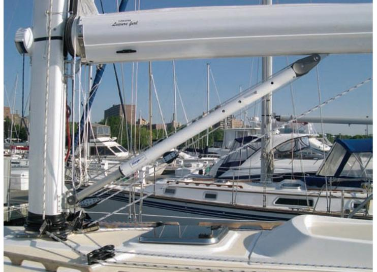
Forespar® makes three sizes of spring loaded boom vang for boats starting around 30 feet and up to about 55 feet. These units are rugged, a good value, and have many thousands of ocean miles under hundreds of boats all over the world. We do not offer the most purchase or have any “locks” or fancy stuff. These are work horses designed to do the job on a general cruising boat or club racer. They will work very effectively if installed correctly and not abused. Some basic points to remember:
