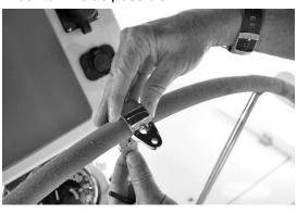
2. Use the 5mm hex wrench to secure the wheel clamp directly to the rim
