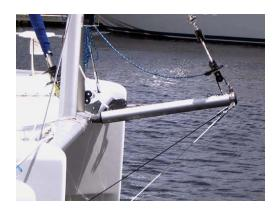
Each sprit pole is specifically sized to match the boat and can be rigged to use with continuous line furling systems or custom
