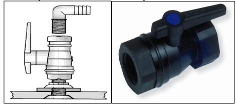
If the valve is installed on the through hull by using a wrench on the top hex nut, the installer can increase the "King" nut pressure on the valve's seals. This will make the handle turn stiff, or seize the valve completely. The problem may not become apparent immediately but the increased stiffness of the handle's operation can cause the handle stem to shear as more force than designed is now required to move the ball.
