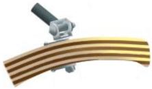
A nylock nut on the set screw which holds the extension to the pin can be tightened down and locked in place at any position. This way the tiller stays at the same angle so that after crossing the boat the sailor is able to reach back and find the extension in the same position he/she left it.
