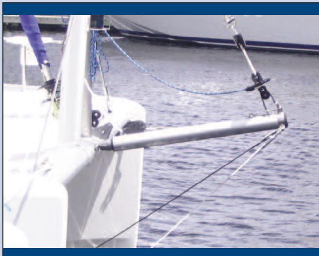
This kit is designed to easily retrofit an existing multihull with no bowsprit to one that has a bowsprit to improve downwind performance using reaching spinnakers and drifter sails.
