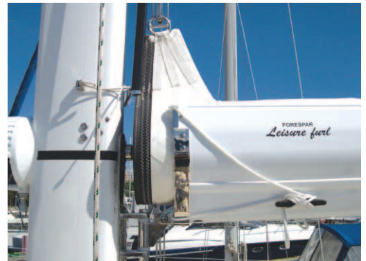
Strong, lightweight polymer luff track with flexible feeder.
