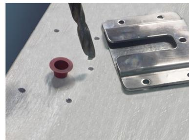
2. Fasten **Fast Kit™** plate to swim step. Insert the bolts provided (or longer, if necessary) and attach them under the swim step with the washers and nuts provided.
