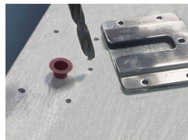
2. Fasten **Fast Kit<sup>™</sup>** plate to swim step. Insert the bolts provided (or longer, if necessary) and attach them under the swim step with the washers and nuts provided.
