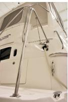
Modular in nature, the rail can be disassembled and stowed in a very compact space. The system comes complete with some fasteners, allen wrench and stainless steel rods. All tubes, rod, terminals and clamps are polished stainless steel.
