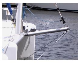
Each sprit pole is specifically sized to match the boat and can be rigged to use with continuous line furling systems or custom configured. Depending on installation, the sprit pole can also be lifted up out-of-the-way or removed.
